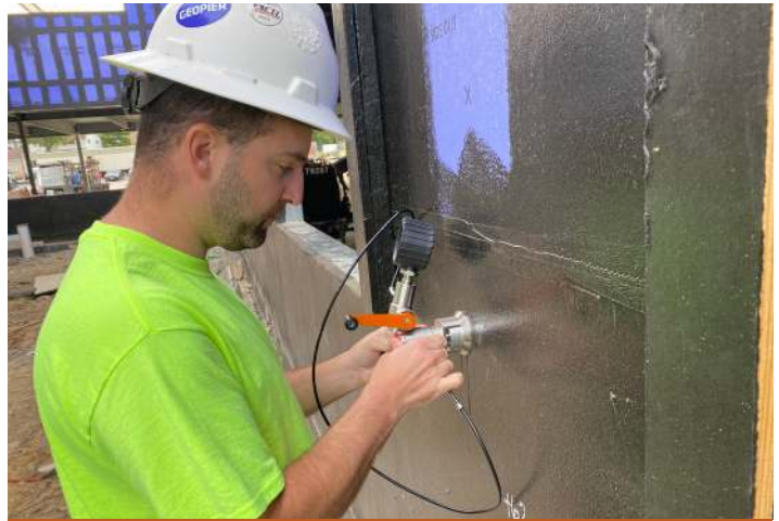
Adhesion testing determines the strength of the bond between substrate and coating or between different coating layers.
