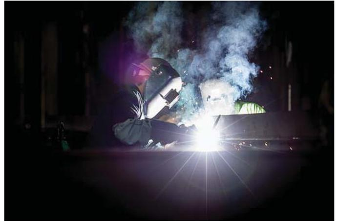
GCI also qualifies welding procedures (WPS) for production companies, fabrication shops and field erection companies. For non-standard welds that are not prequalified in the AWS Standards, regulations dictate a more extensively welded coupon and additional testing procedures.
