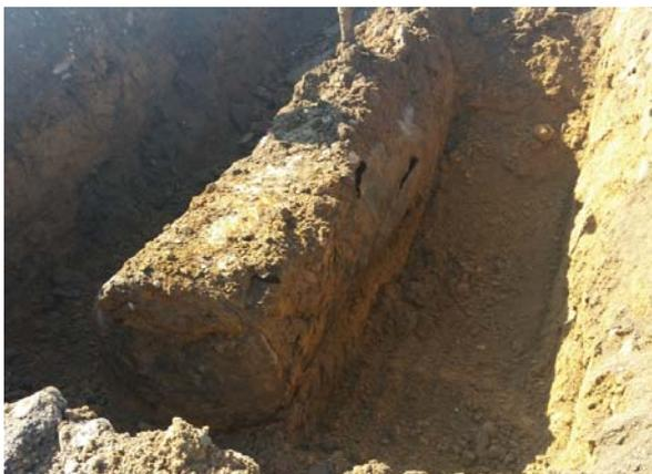
*Older USTs were constructed of bare steel which corrodes over time, allowing liquids to leak into the surrounding soils and possibly contaminate ground water.*
