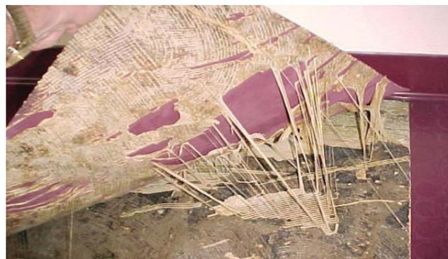
*Adhesive Degradation – Due to excessive moisture and a high pH in the concrete surface, the adhesive under this sheet vinyl has re-emulsified and lost most of its holding strength.*
